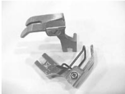
Standard Feet with Needle Guard and Thread Cutter
