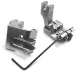
Feet with Double Right Compensating Guide Size Adjustable to: 1/16 & 5/16
