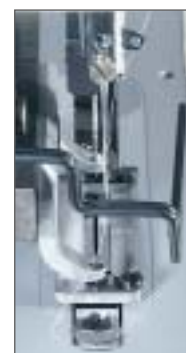
The needle bar can be shifted to the right at the time of threading
