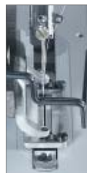
Position of the needle bar during sewing
